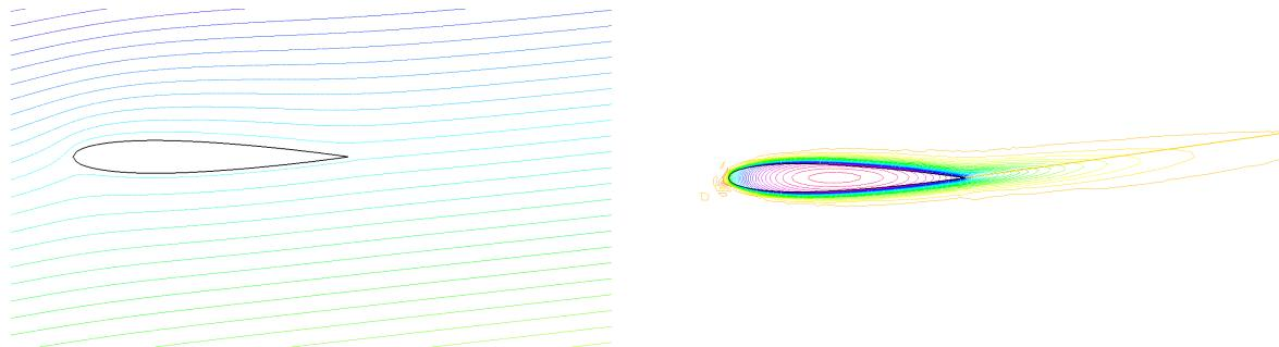
(a) Zoom around the NACA0012 airfoil showing the streamlines (curve  $\psi = \text{constant}$ ). To obtain such a plot use the interactive graphic command: “+” and p.
