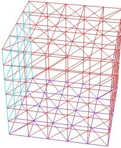
**Fig. 3.23:** The 3D mesh of function `cube(4, 5, 6, flags=3)`
