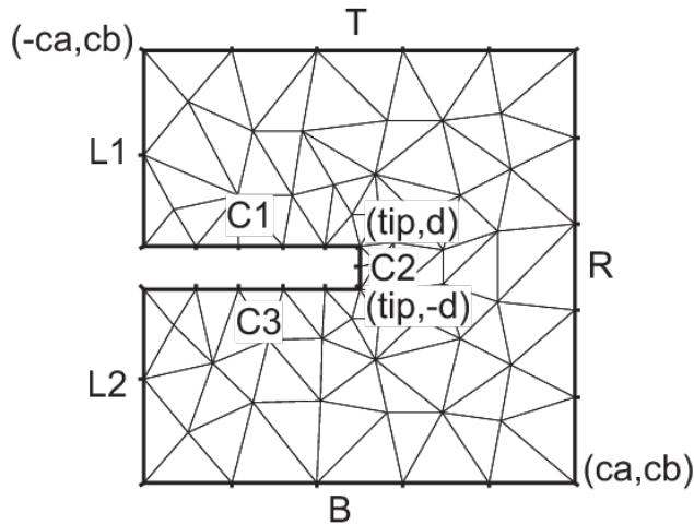
**Fig. 3.19:** Domain with U-shape channel changed by  $d$
