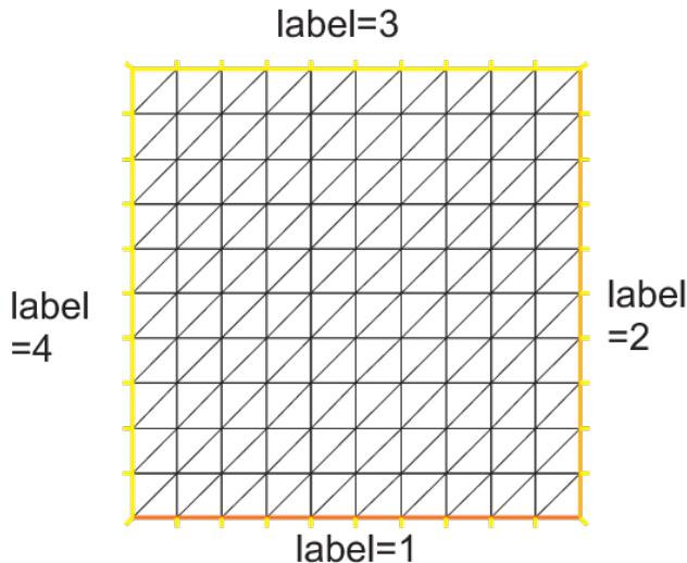
**Fig. 3.1:** Boundary labels of the mesh by `square(10,10)`
