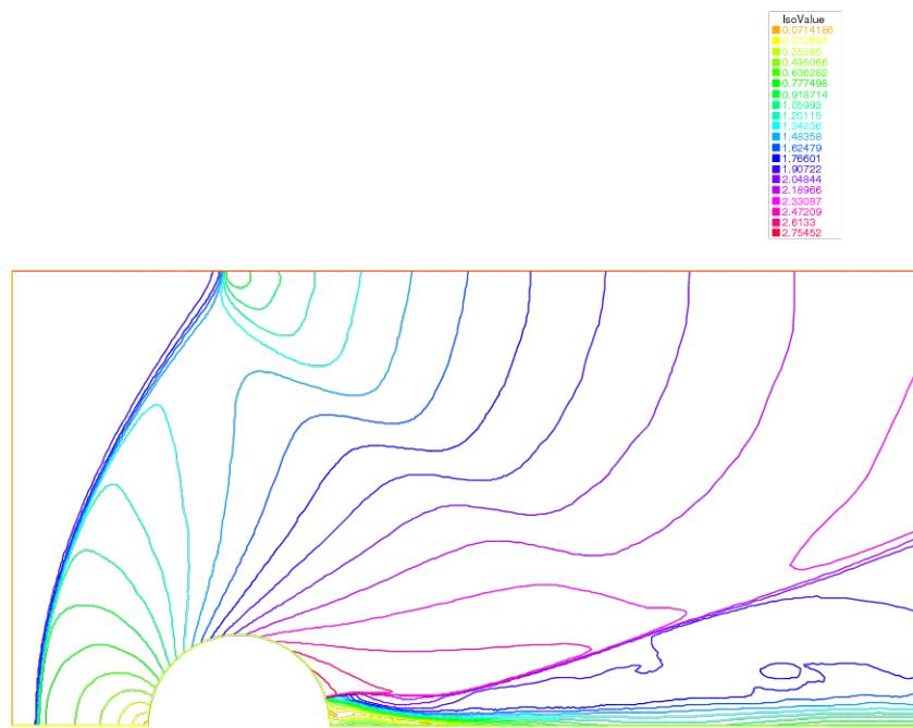
**Fig. 2.18:** Pressure for a Euler flow around a disk at Mach 2 computed by (2.6)
