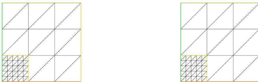
**(a)** Mesh of support the function P1 number 0, split in  $5 \times 5$       **(b)** Mesh of support the function P1 number 6, split in  $5 \times 5$
