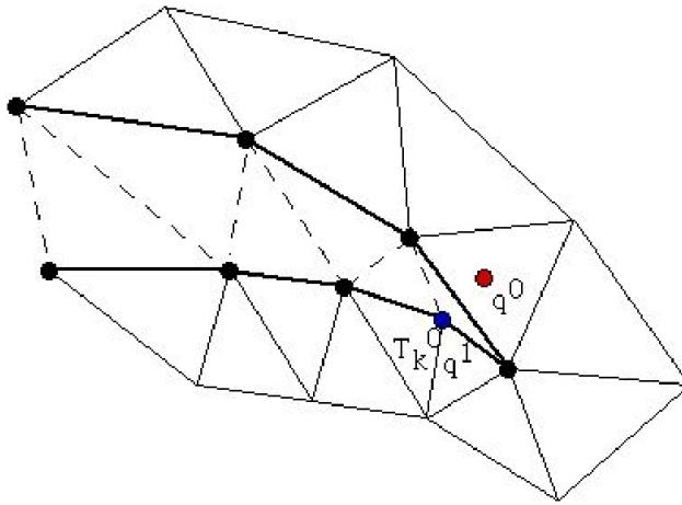
**Fig. 3.37:** To interpolate a function at  $q^0$ , the knowledge of the triangle which contains  $q^0$  is needed. The algorithm may start at  $q^1 \in T_k^0$  and stall on the boundary (thick line) because the line  $q^0q^1$  is not inside  $\Omega$ . But if the holes are triangulated too (dotted line) then the problem does not arise.
