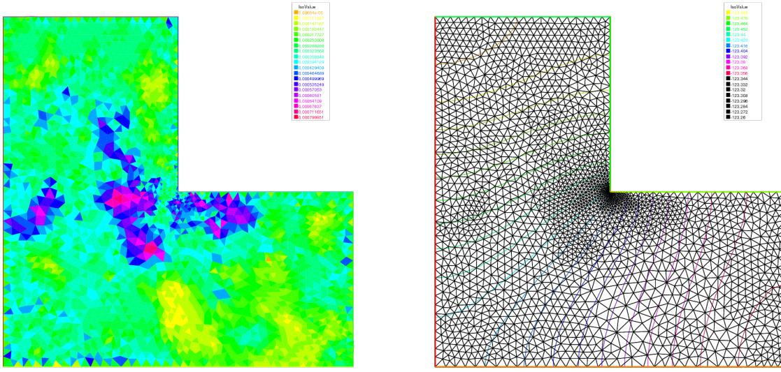
(a) The error indicator with isotropic  $P_1$
