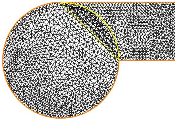
**Fig. 5.18:** The 2 overlapping mesh TH and th
