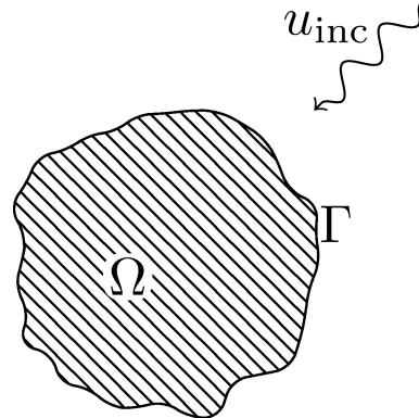
$$\begin{cases} -\Delta u - k^2 u = 0 & \text{in } \mathbb{R}^3 \setminus \Omega \\ u = -u_{\text{inc}} & \text{on } \Gamma \\ + \text{radiation condition} & \end{cases} \quad (3.31)$$
