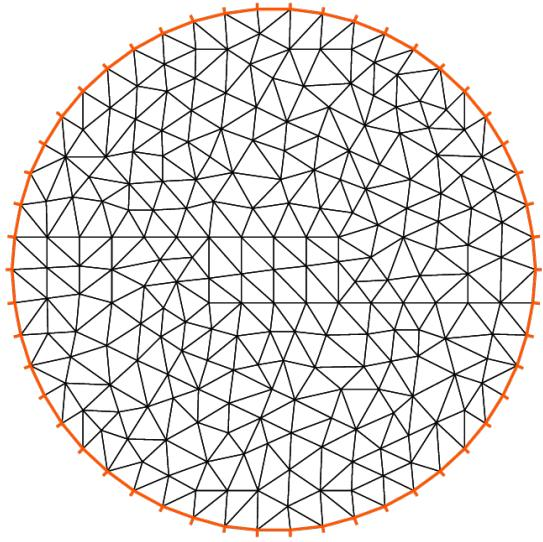
(a) Mesh Th by `buildmesh(C(50))`
