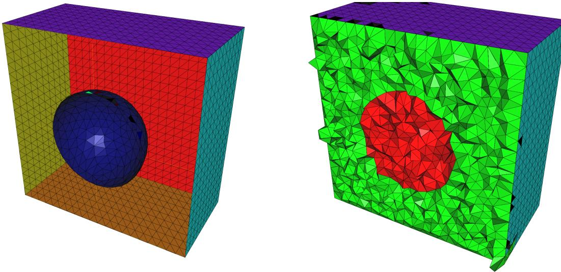
(a) The surface mesh of the hex with internal sphere
