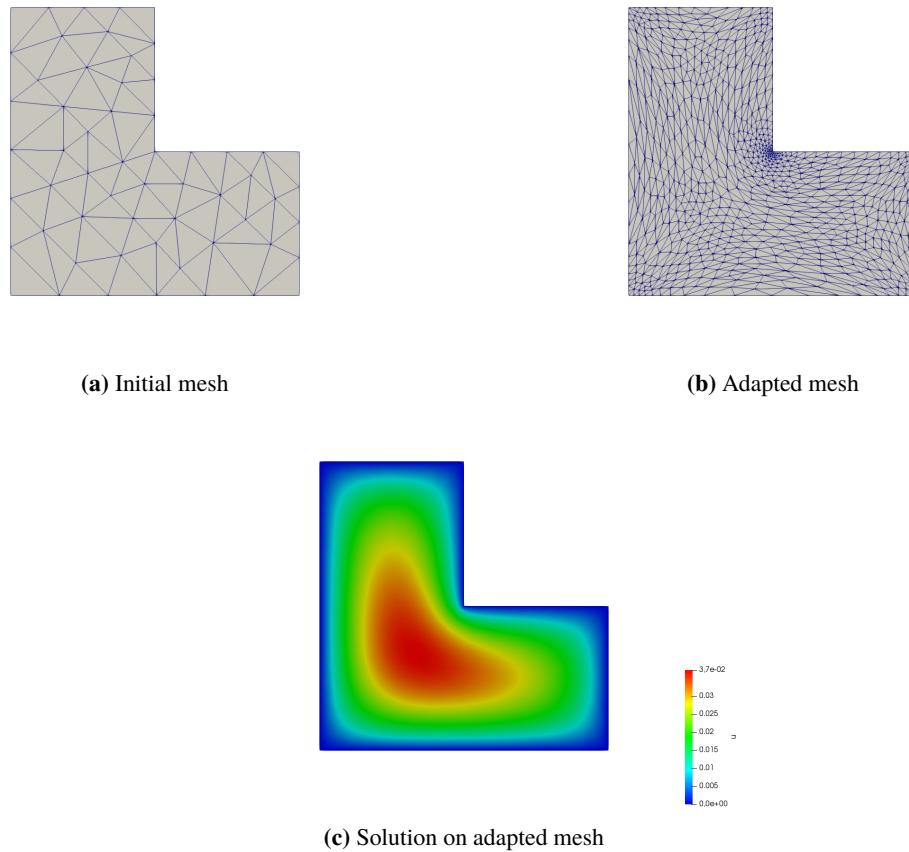
**Fig. 6.5:** Mesh adaptation (Poisson)
