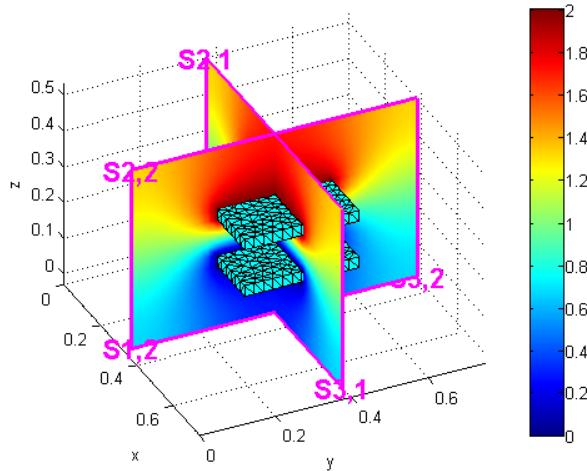
**Fig. 2.27:** Slice on a 3D Parallel Plate Capacitor
