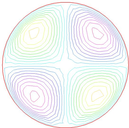
(b) Isovalue by `plot(u)`**Fig. 2.1:** Poisson's equation
