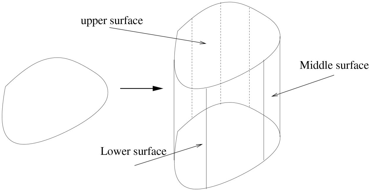
**Fig. 3.24:** Example of Layer mesh in three dimensions.
