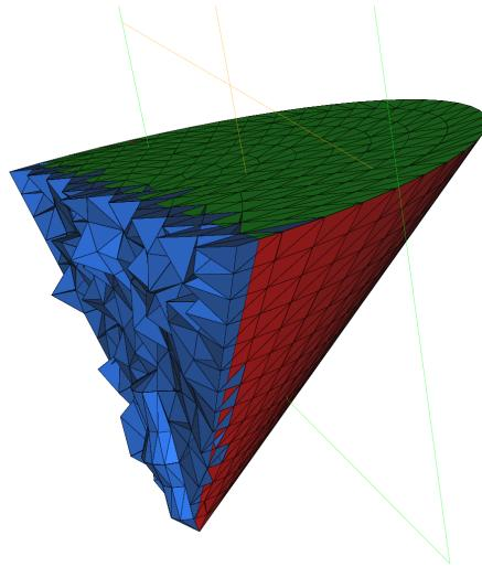
**Fig. 3.26:** The mesh of a cone made with `cone.edp`**Tip:** Buildlayer mesh
