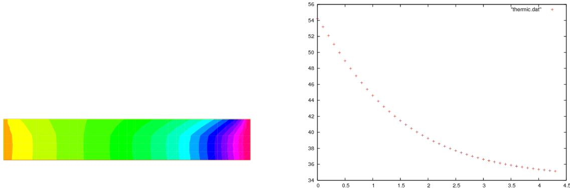
(a) Temperature at  $t = 4.9$ .**Fig. 2.8:** Thermal conduction
