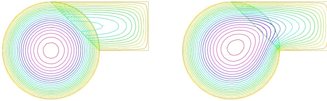
(a) Isovalues of the solution at iteration 0
