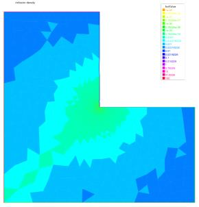
(a) Density of the error indicator with isotropic  $P_2$  metric
