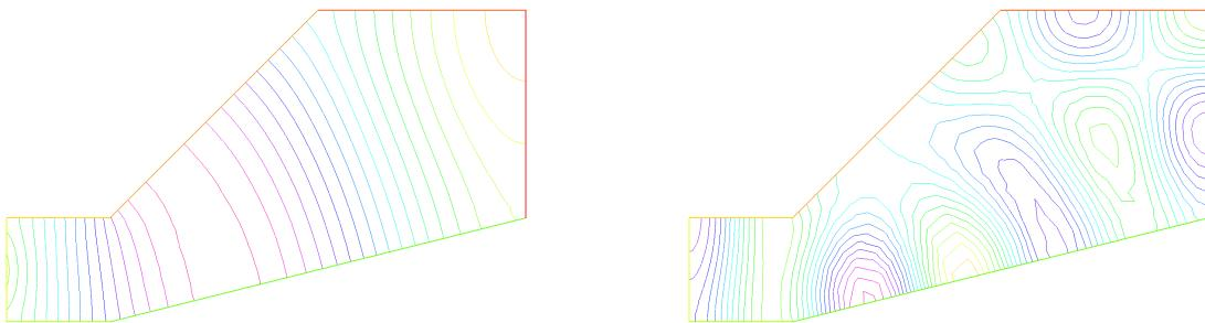
(a) Amplitude of an acoustic signal coming from the left vertical wall.
