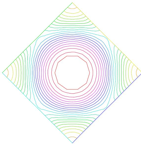
**Fig. 5.6:** The isovalue of solution  $u$  for  $\Delta u = ((y+x)^2 + 1)((y-x)^2 + 1) - k$ , in  $\Omega$  and  $\partial_n u = 0$  on hole, and with two periodic boundary condition on external border
