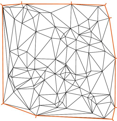
(a) Delaunay mesh of the convex hull of point set in file xy
