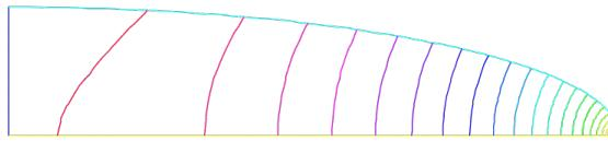
(a) The final solution on the new domain  $\Omega^{7^2}$
